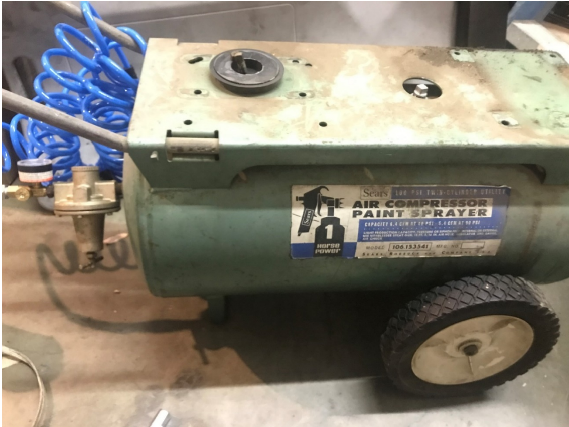
Figure 8.4-2 Air Compressor Tank (Water Tank)
